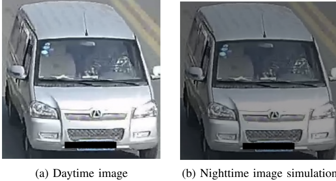
Fig. 5: Simulation of a night image on a day image: night image is obtained by normalizing day image with Day parameters, then scale and shift with Night parameters.
