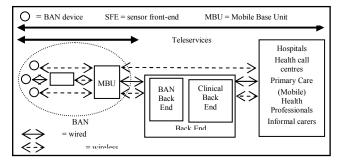
Figure 3. Generic architecture for sensor network systems for m-health
