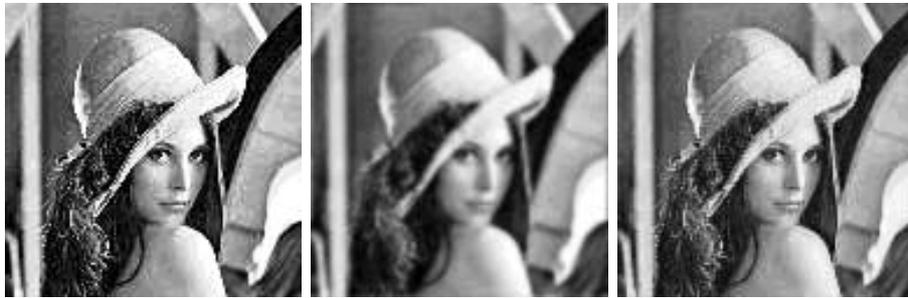
**Fig. 3.** Blind deconvolution result for a 4-bit true image at 70 dB BSNR. (left) True image; (middle) Degraded image; (right) Estimated true image, ISNR 6.12 dB.
