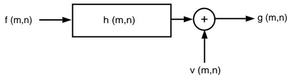
**Fig. 1.** Linear image degradation model.
