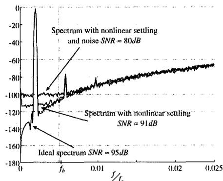
Figure 5. Output spectrum with full scale input.
