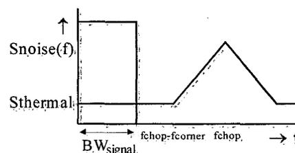
Fig.2: Baseband spectrum at the output
