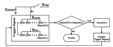
Figure 1. Iterative delay chain discharge method
