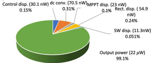
Fig. 9 Power breakdown of the proposed system at frequency of 2 Hz, and voltage output of 1.4 and 4.2 V.
