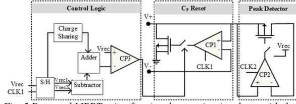
Fig. 5 Proposed MPPT using fractional open-circuit voltage with the waveform.
