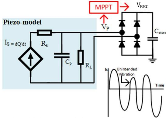
Fig. 2 Simplified circuit model of a PEH energy harvesting system.
