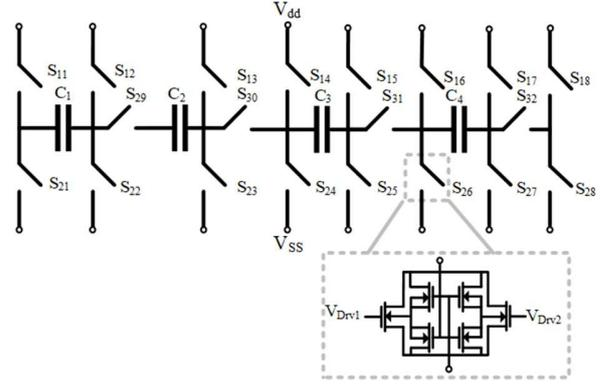
Fig. 6 The 18-Phase switching capacitors with sharing / shorting / recharging phases.
