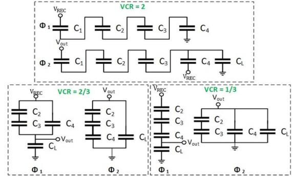
Fig. 7 The buck-boost conversion configurations of the dc-dc converter.
