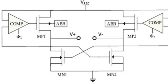
Fig. 4 Proposed SSHC rectifier with PFM control and ABB.
