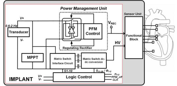
Fig. 3 Proposed PMU design of in-body energy harvesting for post heart implant monitoring.
