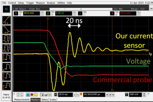
Fig. 7. Detection of a 60-ns current edge.
