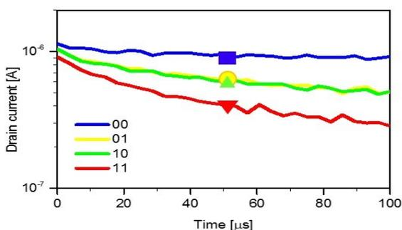
Fig. 6 FTJ measurement showing the possibility of LiM operation. A clear separation of the read currents by a factor of 2 can be observed after a signal development time of  $50\mu$ s as indicated by the symbols.
