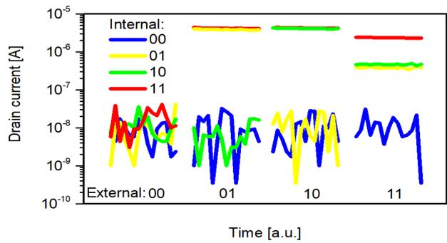
Fig. 5 Result of logic operation between internally stored values in 2 FeCAPs and external input (presence or absence of switching voltage at the corresponding plate line). The measured current levels at SL after applying the switching pulse are shown.
