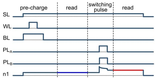
Fig. 2 Pulse waveform used to perform FeCAP read operation (not to scale)
