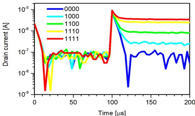
Fig. 4 FeCAP measurement of 4 FeCAPs connected in parallel depending on the stored value.
