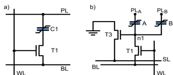
Fig. 1 Circuit diagram of a) FeRAM cell and b) 2T2C cell of this work.
