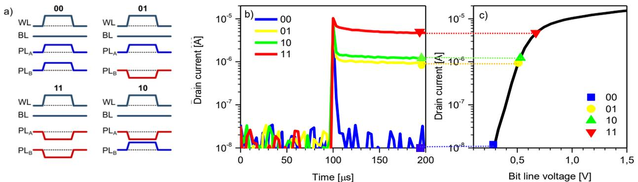
Fig. 3 a) Program pulses used to set the cell into logic states. b) Result of a FeCAP measurement depending on the internally stored value. A clear separation between "00", "01"/"10" and "11" states is observed. c) Id-Vg characteristics of a read-out transistor.
