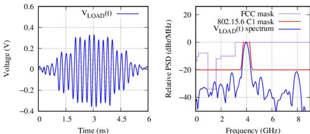
Fig. 8. Pulse for the channel 1 of the IEEE 802.15.6 standard (mandatory).
