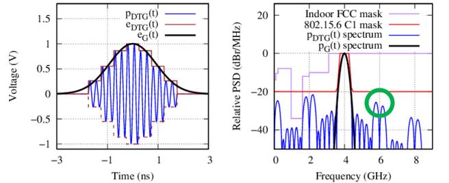
Fig. 3. Example of a pulse with sample & hold Gaussian envelope compliant with the channel 1 of the IEEE 802.15.6 standard ( $K = 7$ ,  $D = 2$ ; the highest sidelobes in adjacent channels are circled in green).
