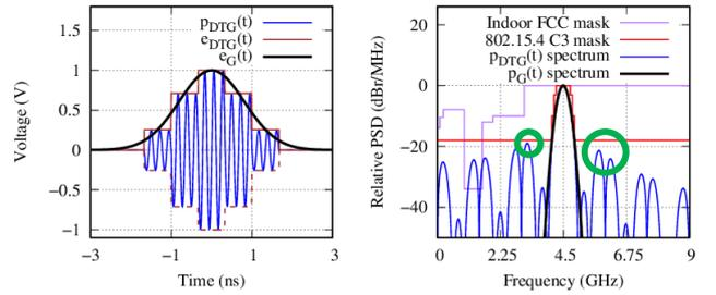
Fig. 2. Example of a pulse with sample & hold Gaussian envelope compliant with the channel 3 of the IEEE 802.15.4 standard ( $K = 5$ ,  $D = 3$ ; the highest sidelobes in adjacent channels are circled in green).
