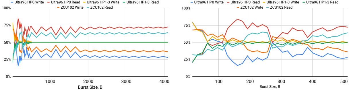
Fig. 5: Measured Read/Write distribution in single AXI base case
