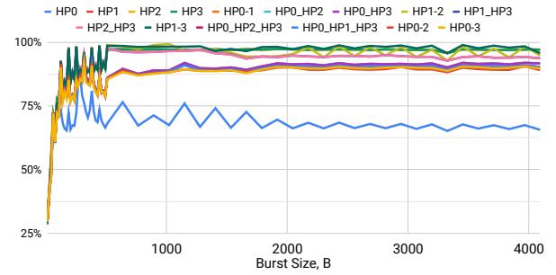
Fig. 12: Throughput of random access pattern on Ultra96 normalised to best results from base case.
