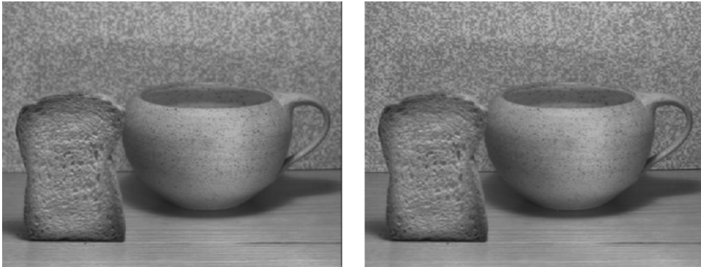
Figure 3. Near-focused original image (left); far-focused original image (right) (courtesy of S.K. Nayar). The difference between the two images is barely perceivable since the two focal planes are only 340 mm apart.
