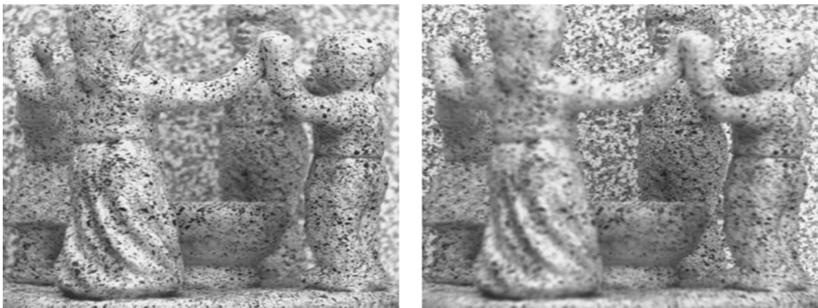
Figure 5. Near-focused original image (left); far-focused original image (right). In this data set the maximum blurring radius is approximately of 5 pixels.
