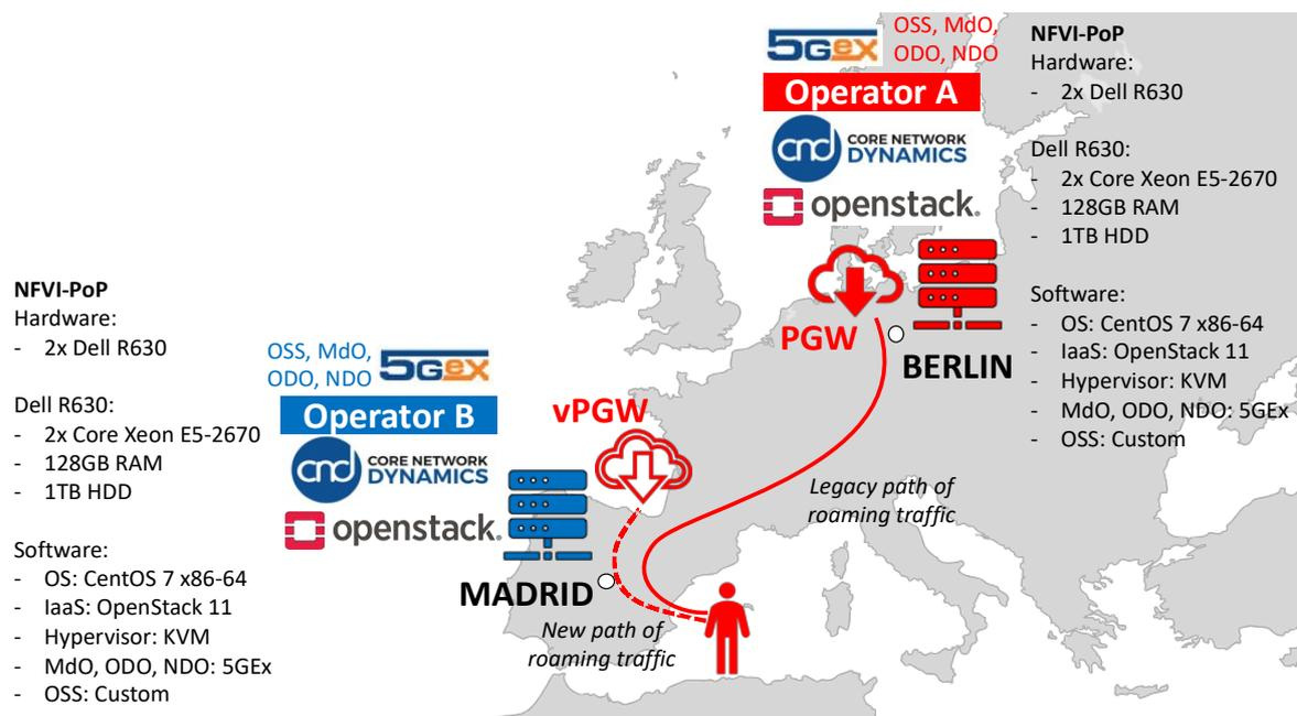
Figure 4-7. Experimental roaming setup consisting of two test-sites: Madrid and Berlin
