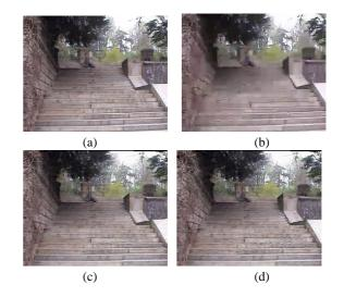
**Fig. 2.** "Thabor" sequence: Image 125 from original sequence (CIF, 25Hz) (a) and reconstructed images at 125kb/s with naive coder (b), with Galpin coder (c) and with our coder (d)
