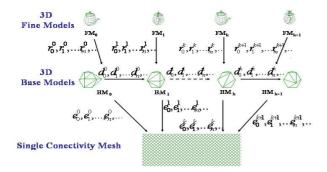
Fig. 1. Proposed representation based on a 3D model stream and second generation wavelets. The fine models  $FM_i$  are represented by the base meshes  $BM_i$  and wavelet coefficients  $r_i^j$ . The scale coefficients  $e_i^j$  expressing the geometry of the base meshes are gathered and indexed by the single connectivity mesh. The meshes are encoded incrementally in time by the wavelet coefficients  $d_i^j$ .
