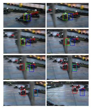
**Fig. 3.** Tracking result of proposed system (red) against SSD (green) and MS (blue) tracker for 'go-carts' sequence. Frames shown 35, 42, 45, 46, 47, 48, 50, 58.
