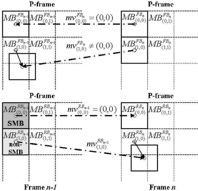
Fig. 2. Macroblock views of the proposed dual-bitstream and the definition of the SMB and non-SMB.
