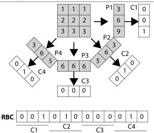
**Fig. 1.** Radon Barcode (RBC) – The image is Radontransformed. All projections (P1,P2,P3,P4) are thresholded to generate code fragments C1,C2,C3,C4. The concatenation of all code fragments delivers the barcode **RBC**.
