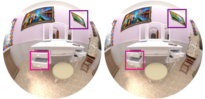
Fig. 1. Block matching between two fisheye images. For visualization purposes, the motion between current (right) and reference (left) frame has been exaggerated.
