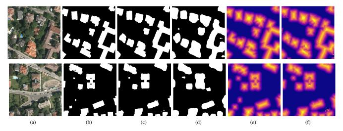
Fig. 4. Two different locations, column-wise: (a) satellite images in RGB, (b) ground truth masks for the building footprints, (c) segmentation predictions by our proposed multi-task network, (d) segmentation predictions by an FCN [5], (e) ground truth masks for distance classes and (f) predicted distance classes. It can be seen that our approach produces less "blobby" predictions with sharper edges compared to the FCN. (Best viewed in electronic version)
