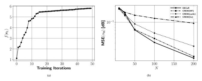
Fig. 2. Illustration of (a) the objective value  $f(s_L)$  of the DECoR vs. training iterations for a code length of N = 10, and (b) MSE values obtained by the different design algorithms for code lengths  $N \in \{10, 25, 50, 100, 200\}$ .
