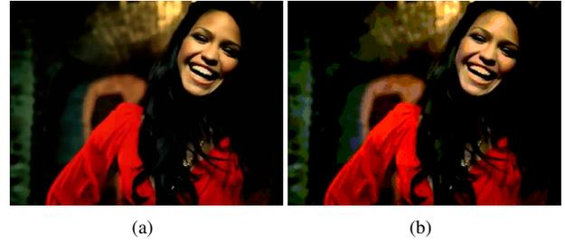
**Fig. 5.** (a) A frame from a testing animated GIF (3.221  $bpp$ ); (b) The same frame after GIF optimization with threshold  $t = 0.125$  (1.3222  $bpp$ ). Although the storage gain is considerable, the quality loss can be visually perceived.
