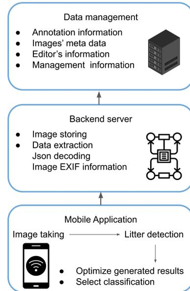
Fig. 1: Architecture for the proposed system for litter monitoring based on a mobile application.
