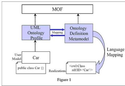
Figure 2: ODM principle
