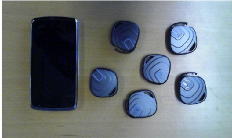
*Figure 2.7. BeSpoon phone and six tags equipped with UWB.*
