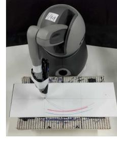
Fig. 7. Touch™ USB haptic devices used during the autonomous operation
