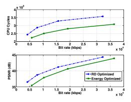
**Fig. 3**. The RD performance and energy saving graphs for the RD optimized bit stream and the energy optimized bit stream.
