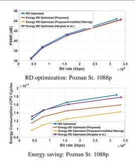
**Fig. 5.** RD and energy saving performance of the proposed energyrate-distortion optimized coding mode selection algorithm.
