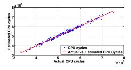
Fig. 2. Actual and predicted CPU cycles per CTU for the Cafe 1080p sequence for QPs 22, 27, 32, 37.
