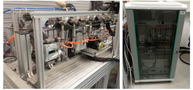
Fig. 4. EHB hardware-in-the-loop experimental setup. On the left, EHB system; on the right dSPACE® box.
