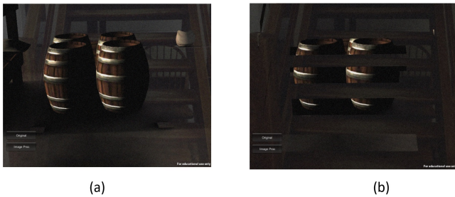
Fig. 6. Handling of static occlusion in the proposed system. (a) Without static occlusion. (b) With static occlusion.
