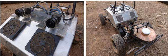
Fig. 3. Platform sensors connected to the on-board computer. *Left*: Two vision cameras, 1280x1024, 70fps, global shutter, synchronously triggered. *Right*: RTK-corrected Hemisphere Eclipse P307 GPS module, position at 20Hz.
