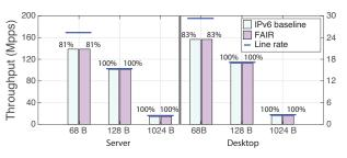
Fig. 10: Switching performance of the server and the desktop for all ports activated, and 68, 128, and 1024-byte packets.
