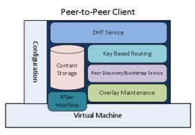
Fig. 2. Architecture of a P2P client in the VPN overlay
