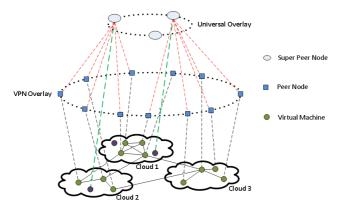
Fig. 1. Two-tiered architecture for the Inter-Cloud VPN solution
