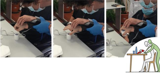
Fig. 4. Stroke patient executing grasping tasks using the EMG-controlled SoftHand-X during the experimental phase. The physiotherapist supports the arm and forearm, helping the patient in the proximal movements.
