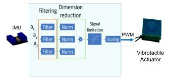
Fig. 2: Control strategy diagram of the vibrotactile system. The acceleration signals acquired from the IMU (left) undergo a signal elaboration process (filtering, dimensional reduction, and other minor elaboration steps). The processed signals are encoded into a PWM signal and transmitted to the actuator (right).
