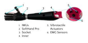
Fig. 6: The VIBES integrated inside the prosthesis. A detailed view (right) shows the inner part of the socket with vibrotactile actuators and EMG sensors.
