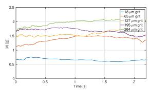
Fig. 4: Sandpaper acceleration signals: acceleration module  $|\mathbf{a}|$  recorded for each sandpaper type.
