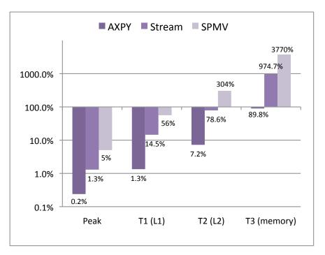
Figure 4: Efficiency estimates based on peak performance values and several statically computed predictions (for a fixed problem size): ratio of predicted time vs. measured time.
