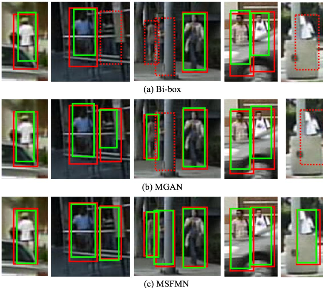
Fig. 6. Qualitative detection comparison of (a) Bi-box [7], (b) MGAN [9] and (c) MSFMN under different occlusions on caltech test images. All detection results are obtained using the same false positive per image criterion. The solid red boxes denote the ground-truth, dashed red boxes represent the missed detections and the green boxes present detection results. For better visualization, the detected regions are cropped from the corresponding images.
