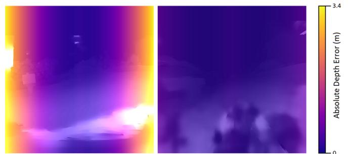
Fig. 5: Absolute Depth Error (m) overlain onto disparity maps generated using Mei-Rives (left) and Scaramuzza-Urban (right) with SGBM-WLS stereo disparity estimation .
