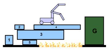
Fig. 1. An example of a robotic agent having designed and built a stable structure to climb the obstacle G and avoid the hazardous flaming region. Objects  $o_1$ ,  $o_3$  and  $o_5$  have 2 units of mass, where objects  $o_2$  and  $o_4$  have 6 and 3 units. The robot weighs 0.5 unit.
