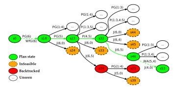
Fig. 4. The planning graph for the simple example where the green arrows represent the desired plan and the state *s*53 satisfies the goal requirements.
