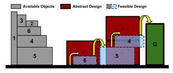
Fig. 3. The final result of a simple problem of obstacle climbing. The yellow 'right-turn's represent the actions 'WalkFromGround' and 'WalkAbove', and the 'u-turn's represent the 'Jump' actions.
