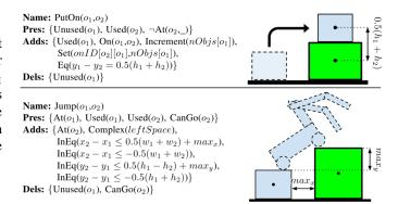
Fig. 2. The example definition for two actions,  $PutOn(o_1,o_2)$  and  $Jump(o_1,o_2)$ , which put one object on another and drive the robot over a gap between two objects, along with their effects in the environment.
