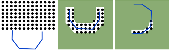
Fig. 2: We can think of tactile localization as a problem of set cover, which is adaptive submodular [23]. Each observation amounts to covering (green area) the hypotheses (black dots) which do not agree. Our objective is to maximize our coverage, or rule out as many hypotheses as possible.
