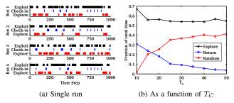
Fig. 5. Time spent in each control mode, Exploit (black), Check-in (blue), and Explore (red). (a) The time evolution of the mode switching for each individual robot over an example run. (b) The fraction of the total time spent in each mode as a function of  $T_C$ .
