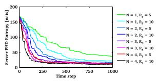
Fig. 4. Time evolution of the entropy of the target RFS for a variety of team sizes and footprint radii.
