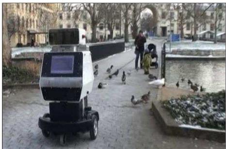
Fig. 10. Dynamic 3D obstacles which pose substantial challenges for the navigation system.
