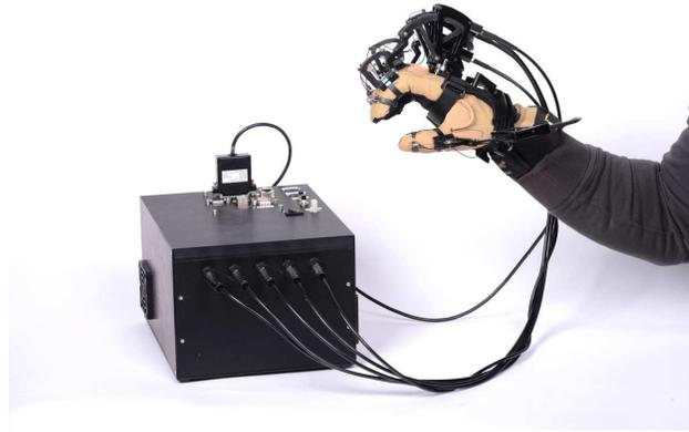
Fig. 1. The ExHand Box with CyberGrasp<sup>TM</sup> and CyberGlove<sup>®</sup> connected. The only external interface required is power through a laptop-like supply.
