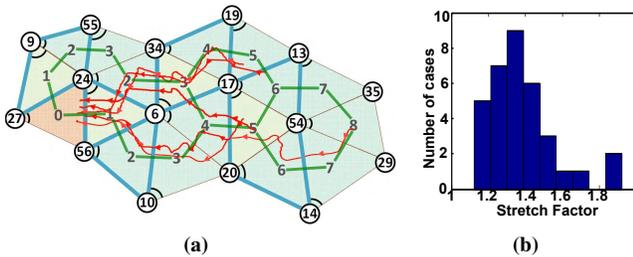
Fig. 11: (a) Sample navigation results with 12 robots. (b) Stretch factor histogram with 34 trials of navigation experiment.
