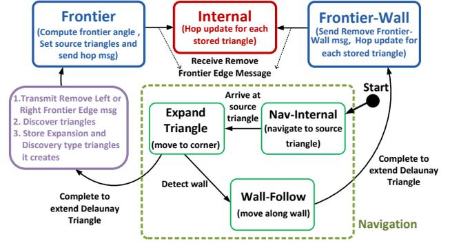
**Fig. 6:** Finite state machine for MAT algorithm.
