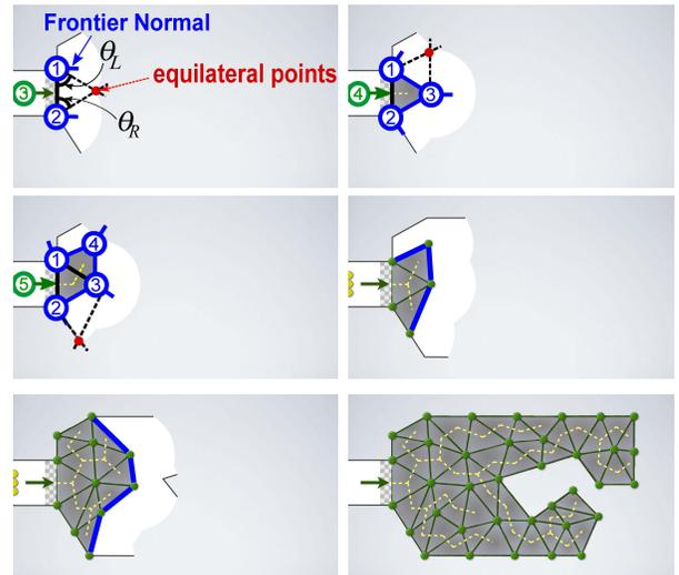
**Fig. 3:** Constructing a triangulation in a BFS manner. The frontier edges are blue and interior edges are green. The edges of the BFS tree (the dual graph) are yellow. The blue tick marks on each robot show the direction of the *frontier normal*. This points into unexplored space, in the direction perpendicular to the frontier edges incident at each robot.
