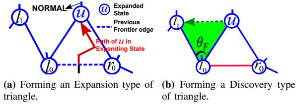
**Fig. 4:** (a) An example of *Expansion* triangle: Red arrow is the path of  $u$  in *Expanding* state. After arriving at the equilateral point,  $u$  switches to *Expanded* state. (b) An example of *Discovery* triangle (light green).  $u$  checks  $\theta_F$  to evaluate the quality of candidate triangle,  $\Delta u l_1 l_0$ .
