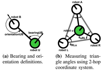
**Fig. 2:** (a) Robot  $u$  can measure the bearing to neighbor  $u_L$ ,  $B_u(u_L)$ , and the orientation of neighbor  $u_L$ ,  $Ori(u_L)$ . (b), triangle angles (black arrows) are measured from neighbors of robot  $u$ , and shared with  $u$  using a local broadcast message. We define left (right) inner angle for the triangle angle of  $u$ 's left (right).
