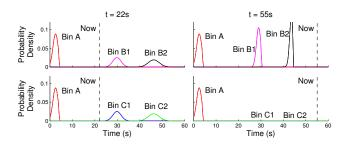
Fig. 6: Inference result at two different times where the human reaches into bins A, B1, and B2. As more evidence is observed, the robot understands that the human does not need C1 or C2 and the timing predictions become sharper.
