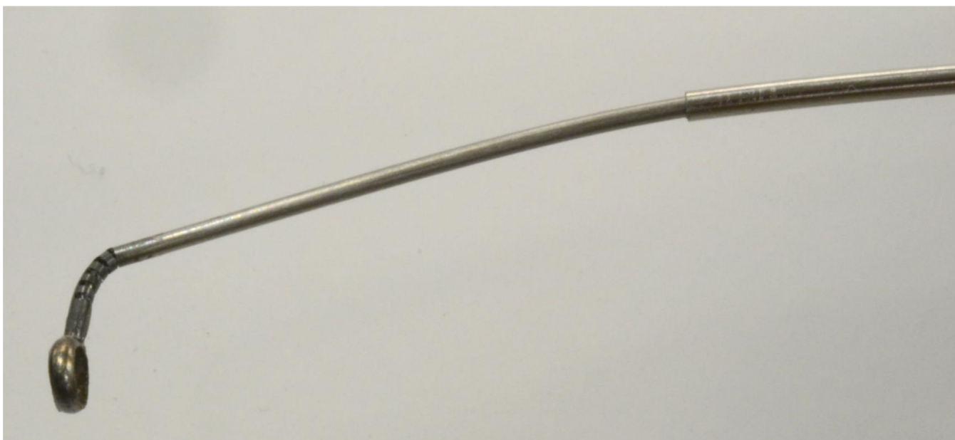
Figure 1. Photograph of a wrist mounted to the tip of a concentric tube robot. The diameter of the wrist is 1:16 mm.
