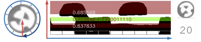
Fig. 7. Histogram for an unrolled circular marker and rotation invariant binning of the code stripe. The numbers from top to bottom indicate the probabilities for center, binary code and outer circle. The marker with ID 20 has been successfully decoded.
