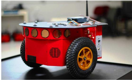
Figure 1: Mobile robot based experimental platform (Pioneer 3 DX) with two-wheel differential and caster.
