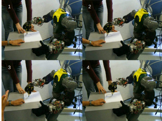
Fig. 6: COMAN performing a drawing task on a desk, interaction is handled by joint impedance control
