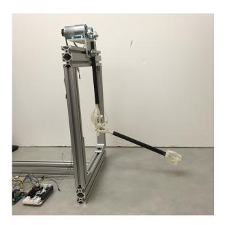
Fig. 9. The physical prototype of our tensegrity elbow. Compression elements are composed of 3D-printed Polylactic Acid (PLA) and tension elements are composed of spectra braided fishing line. This model is actively controlled by motors seen mounted off of the robot and onto the chassis.
