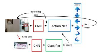
Fig. 8. Overall architecture of our active recognition system. It consists of three components. A CNN for extracting image features from the entire image given the current view, an instance classifier for classifying the cropped object, and an action network for selecting the next action in order to improve classification.
