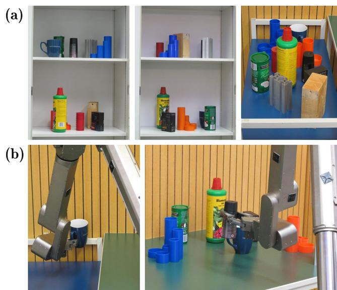
Figure 7: (a) Start configurations used for the grasping trials with randomly placed set of objects. (b) Example of a pick operation (left) and a place task (right).
